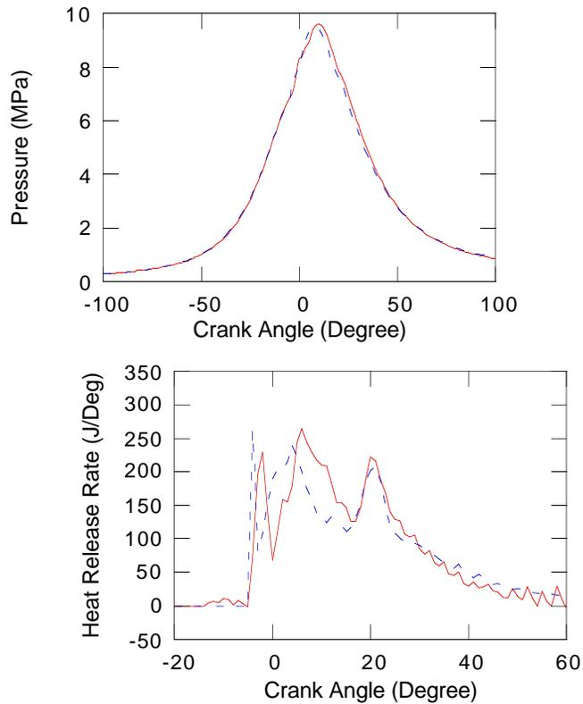
**Figure 9** Pressure and heat release rate predictions for split injections. The dwell between the two injection pulses is eight degrees. Solid line--measured, dash line--predicted. From top: 10-8-90, 25-8-75, 50-8-50 and 75-8-25.
