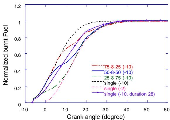
**Figure 12** Fuel burnt histories showing combustion evolution. The burnt fuel is normalized by the total injected fuel.
