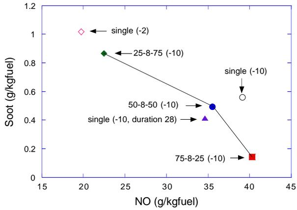
**Figure 13** Computed soot-NO trade-off of the designed injection schemes.
