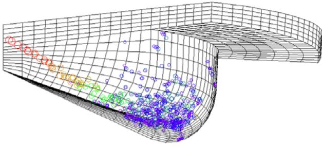
**Figure 1** Outline of the computational mesh at TDC. Spray droplets (circles) are superimposed for reference.
