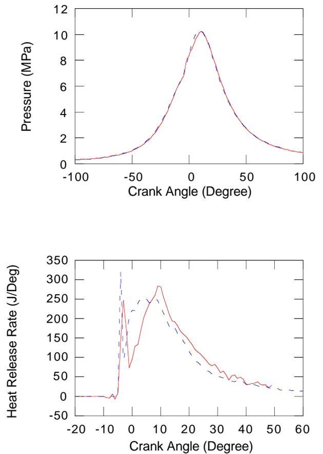
**Figure 7** Single injection predictions. Spray injection timing is 10.5 degrees BTDC. Solid line--measured, dash line--predicted.
