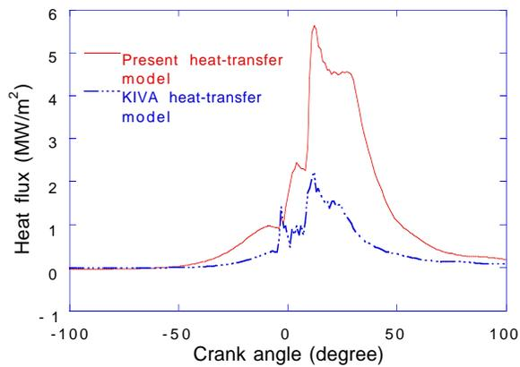
**Figure 4** Predicted wall heat fluxes. The monitoring location is over the piston bowl at the edge of the bowl at the cylinder-head surface in the plane of the spray.
