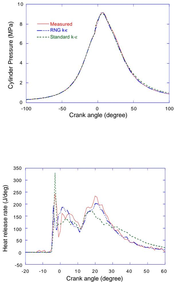
**Figure 3** Effect of turbulence model on combustion prediction.
