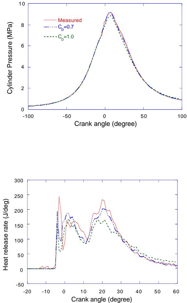
**Figure 6** Effect of nozzle discharge coefficient on combustion prediction.
