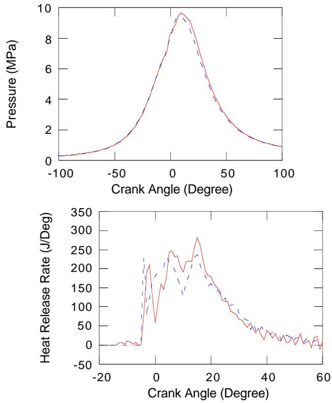
**Figure 8** Pressure and heat release rate predictions for split injections. The dwell between the two injection pulses is three degrees. Solid line--measured, dash line--predicted. From top: 10-3-90, 25-3-75, 50-3-50 and 75-3-25.
