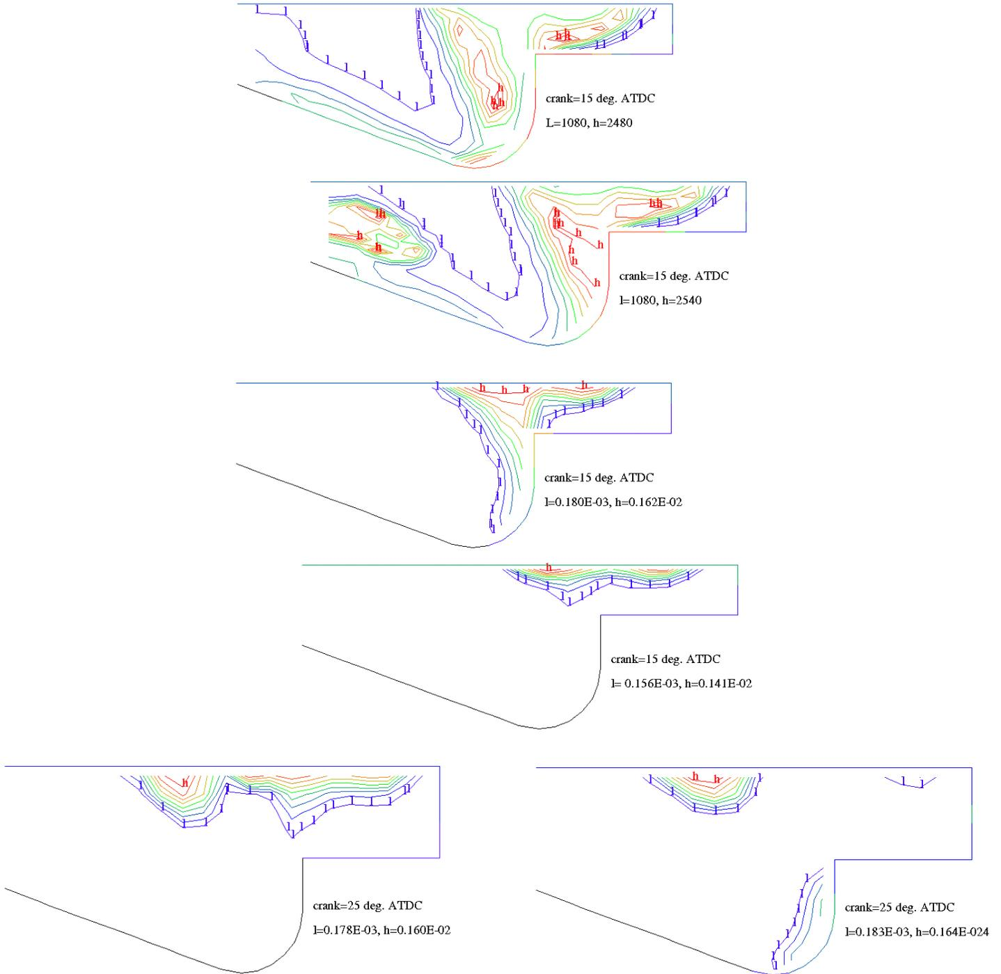
**Figure 21** Computed temperature (K) (top) and soot concentration ( $\text{g}/\text{cm}^3$ ) (middle and bottom) contours in the plane of the spray axis. Left: Single injection (-10). Right: Split injection 75-8-25 (-10).
