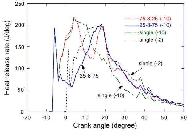
**Figure 15** Computed heat release rates for the single and double injection schemes.
