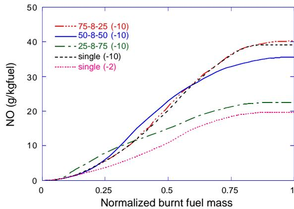
**Figure 14** NO formation history as the function of burnt fuel mass. The burnt fuel is normalized by the total injected fuel. The single injection cases have a 20-degree duration.
