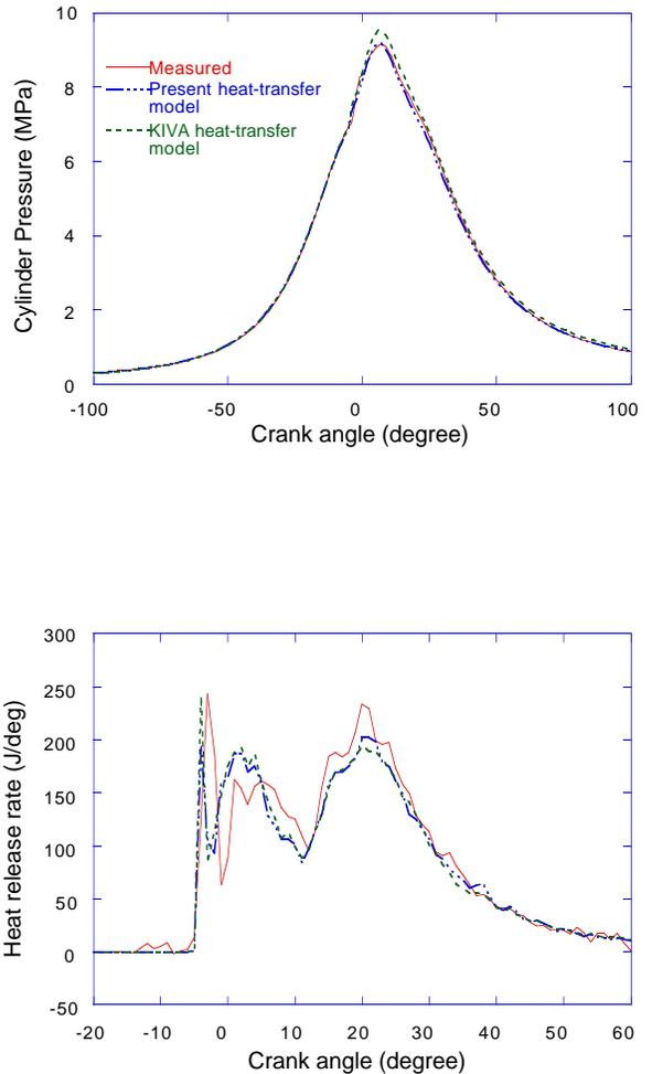
**Figure 5** Effect of gas/wall heat transfer model on combustion prediction.
