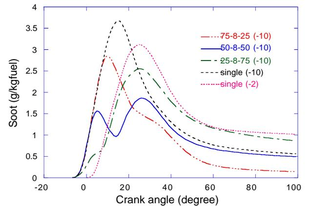
**Figure 17** In-cylinder soot production history for single and double injection schemes.
