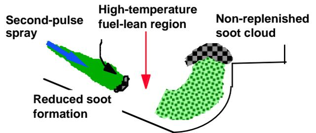
**Figure 20** Schematic diagram showing soot-reduction mechanisms of split injections. Left: Single injection. Right: Split injection.
