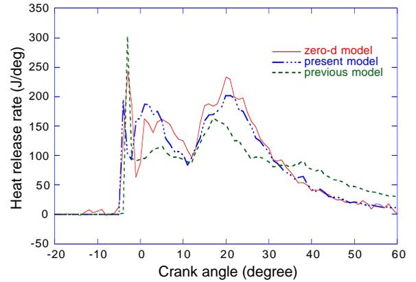
**Figure 2** Comparison showing improvements in multiple-injection combustion predictions using the present model.
