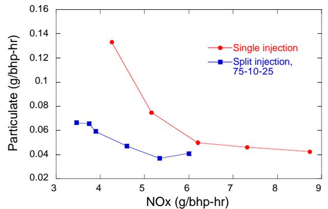
**Figure 23** Measured particulate-NO<sub>x</sub> trade-off of a Caterpillar engine at 75% load for single and double injections [3]. Injection timings were varied from -12 to +1 ATDC.
