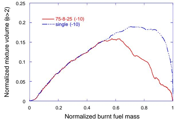
**Figure 19** In-cylinder rich mixture volume normalized by the instantaneous total volume showing the effects of the second-pulse injection on fuel/air mixing.
