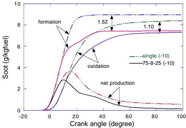
**Figure 18** In-cylinder histories of soot formation, oxidation and net production.
