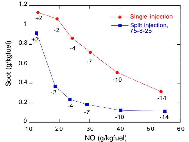
**Figure 22** Computed soot-NO trade-off showing predicted emission reduction using split injections. Numbers in the figure are the injection timings (ATDC).
