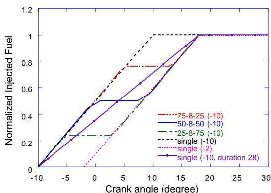
**Figure 11** Injected fuel as function of crank angle. The injected fuel is normalized by the total injected fuel.
