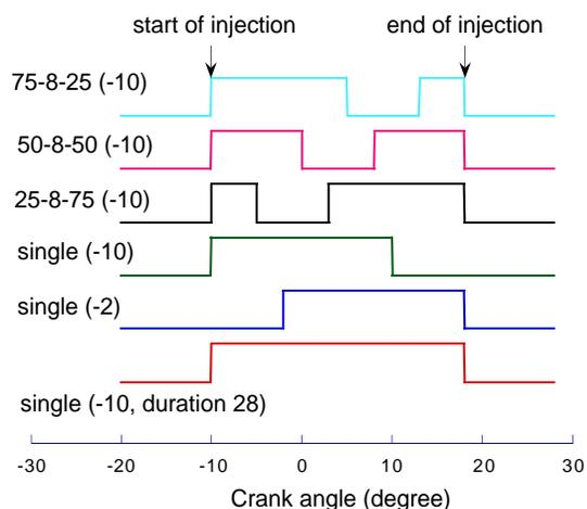
**Figure 10** Schematic showing model injection schemes.
