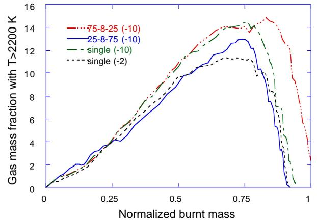
**Figure 16** In-cylinder high-temperature mixture fractions. The burnt fuel is normalized by the total injected fuel.
