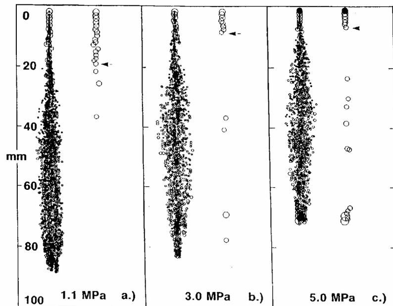
**Fig. 3.12** Spray parcel plots showing co-existing large drops and small product drops in the core region near the nozzle. Plots at the right show only the parcels containing drops with diameters larger than 180  $\mu\text{m}$  (Reitz, 1987).
