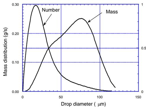
**Fig. 3.1c** Measured total spray drop size distribution 50 mm downstream of nozzle exit.
