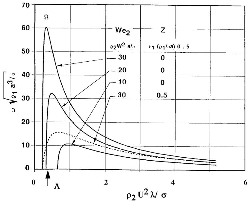
**Fig. 3.4** Wave growth rate versus wave number as a function of Weber number and Ohnesorge number. The maximum wave growth rate and length scale are  $\Omega$  and  $\Lambda$ , respectively.
