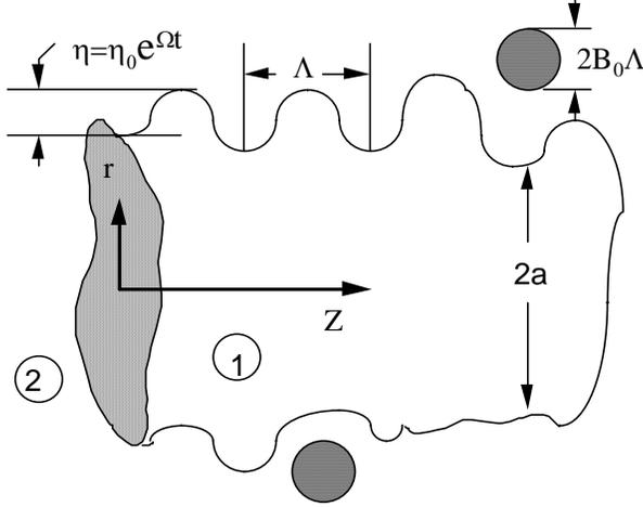
**Fig. 3.3** Schematic diagram showing surface waves and breakup on a liquid jet or "blob".
