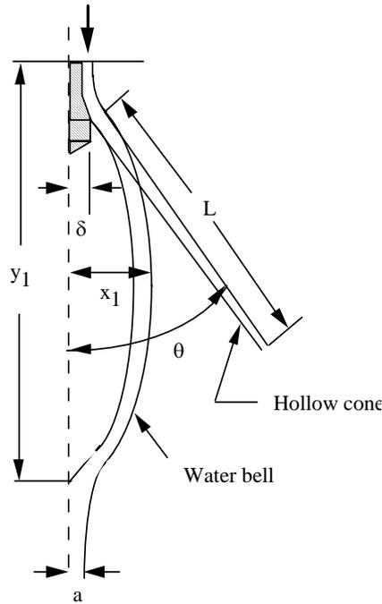
**Fig. 3.9a** Poppet nozzle sheet breakup schematic diagram
