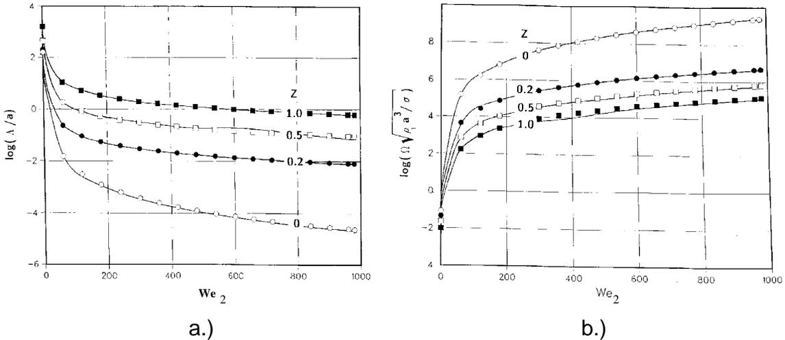
**Fig. 3.5** Wavelength a.) and growth rate b.) of the most unstable surface wave versus Weber number,  $We_2$ , as a function of Ohnesorge number,  $Z$  (Reitz, 1987).
