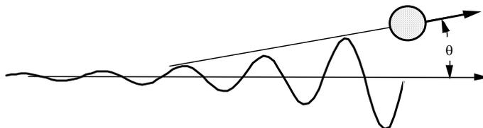
**Fig. 3.7b** The spray angle,  $\theta$ , is determined from the wave growth rate by injecting drops with a normal velocity component,  $v$ .
