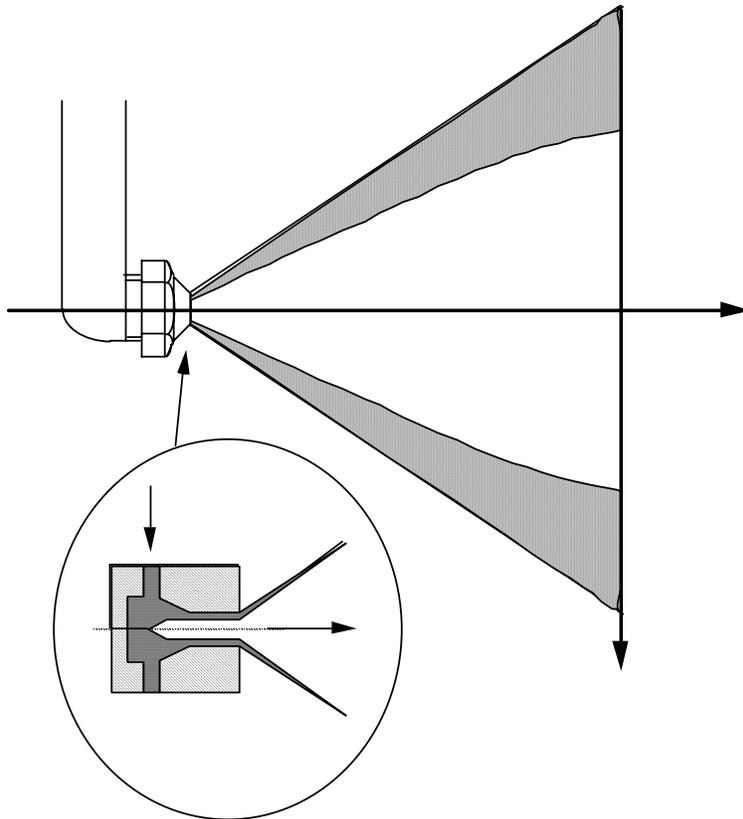
**Fig. 3.1a** Pressure atomized hollow-cone spray nozzle of Dodge and Schwalb (1989).
