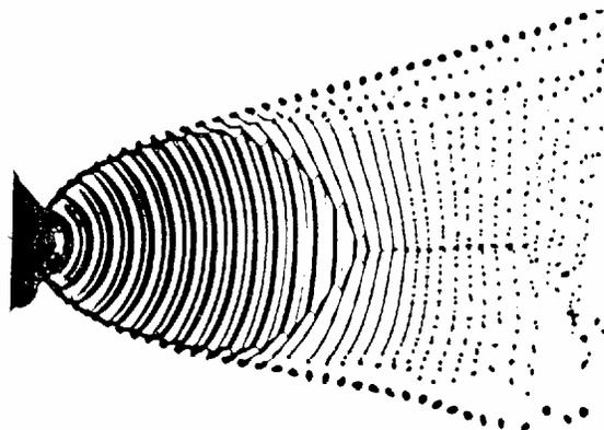
**Fig. 3.8b** Induced breakup of a liquid sheet from a perturbed fan-spray nozzle (Van Dyke, 1982).
