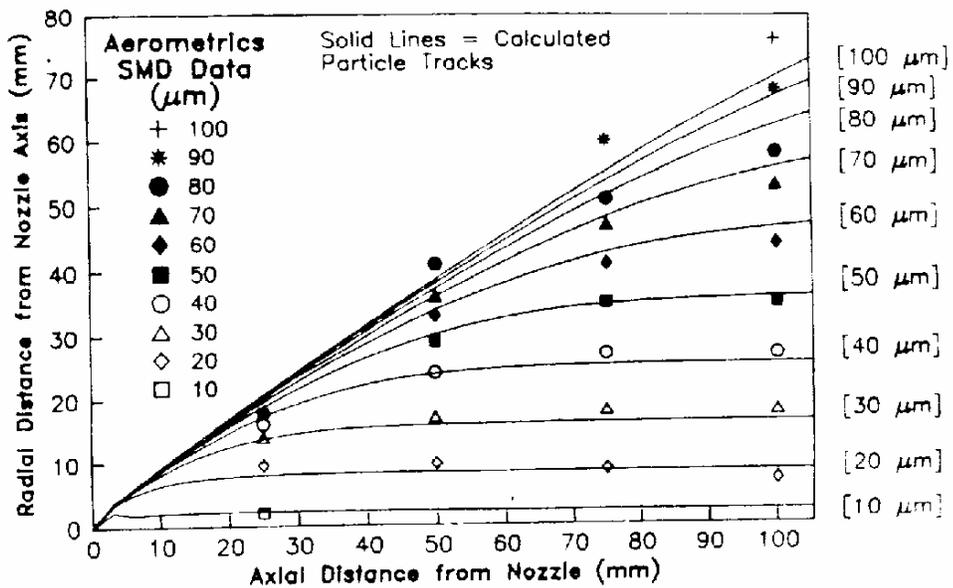
**Fig. 3.1b** Comparison of drop trajectories measured and predicted by FLUENT of Dodge and Schwalb (1989).
