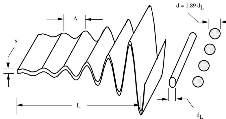
**Fig. 3.8a** Breakup mechanism of liquid sheets.
