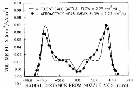
**Fig. 3.1d** Comparison of measured and predicted volume flux distributions 50 mm downstream of nozzle exit.
