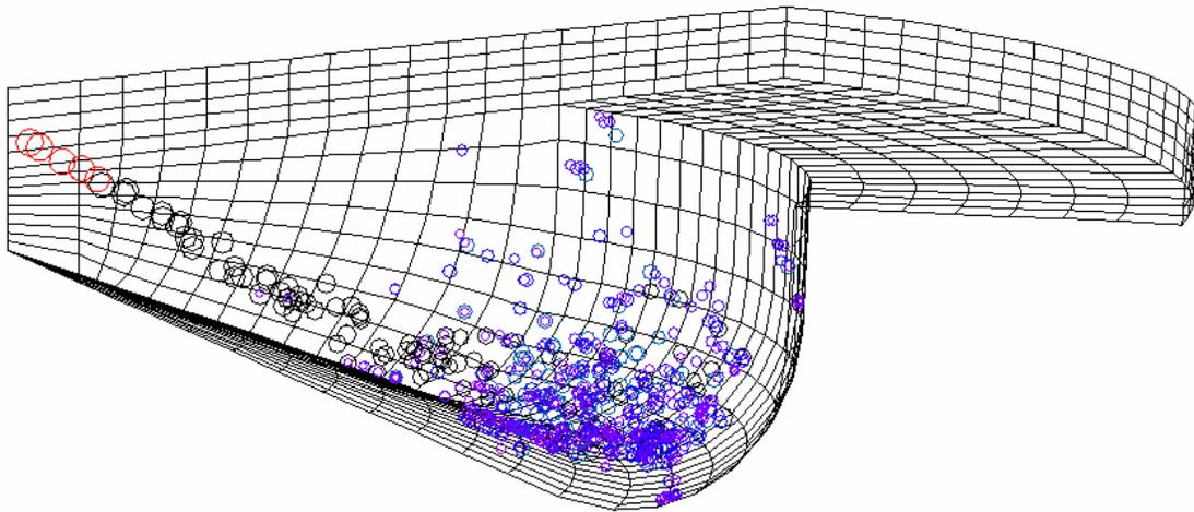
**Fig. 3.13** Computational mesh showing spray parcel locations at 5 degrees after top-dead-center in a diesel engine. The spray impinges on the surface at the bottom of the piston bowl. A core region of large drops is seen near the nozzle (top left) (Patterson et al. 1994).
