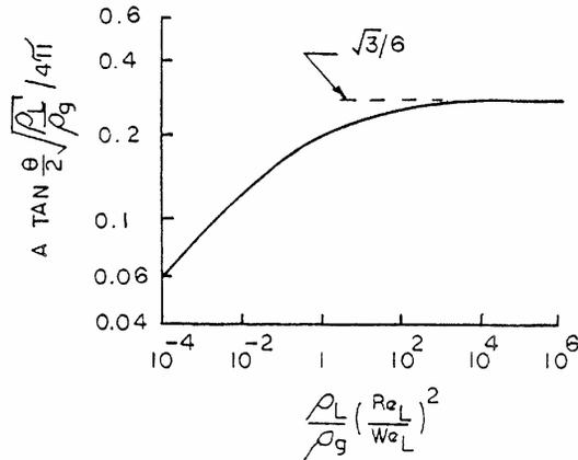
**Fig. 3.7a** Theoretical dependence of the spray angle parameter  $f(T)$  on Taylor's number  $T = \rho_L / \rho_g (Re_L / We_L)^2$  (subscripts L and g refer to the liquid and gas phases, respectively).
