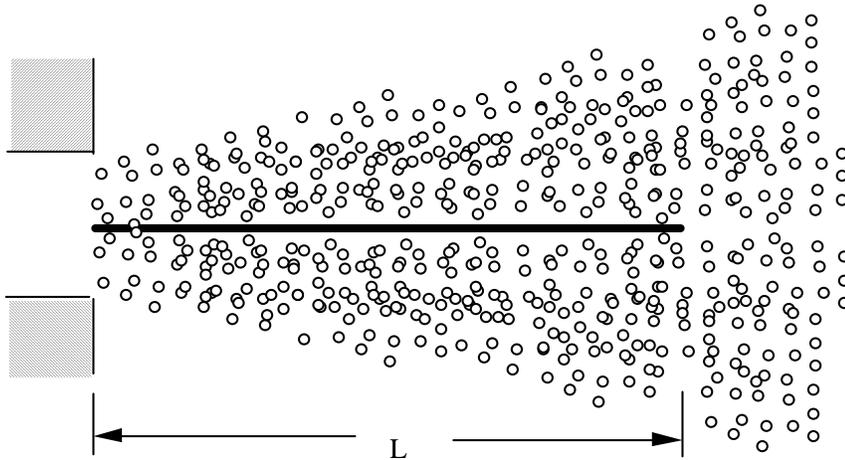
**Fig. 3.6** Line-source atomization model (Chatwani and Bracco, 1985).
